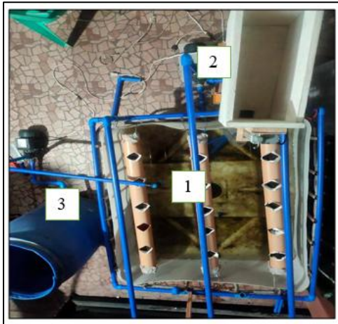
Figure 9. Top View 1- Aquaponics system, 2 – feeding system, 3 – water system
