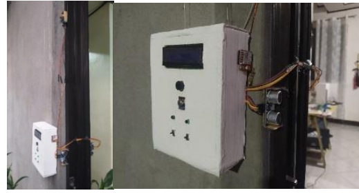
Figure 2: Crowd Entry Limiter Life Sized Door Model
